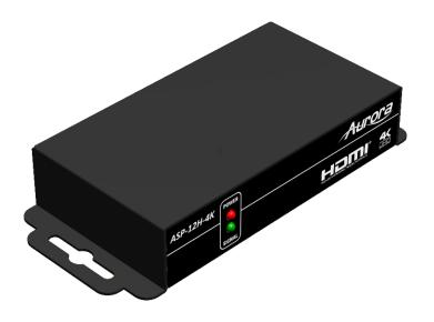
The **ASPYRE HDMI 4K2K Splitter Series with EDID Management** provides one of the most advanced HDMI splitter solutions by which the Ultra High Definition video and high quality audio can be transmitted to multiple locations without losing quality. The series supports all 3D formats and true 4K2K video. Available in 1x2, 1x4, and 1x8 configurations.
